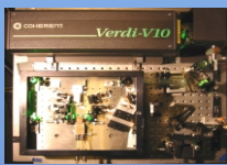
(a) highly compact Ti:sapphire laser (GigaJet 20, GigaOptics GmbH) modified to support higher spectral bandwidth
